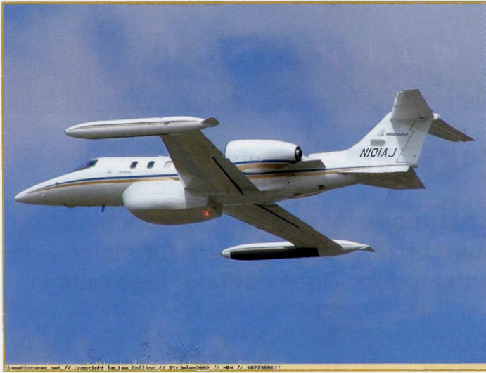
Intermap's STAR-3i Interferometric Radar (IFSAR) mapping system collects a swath width of 9-kilometres from a flight altitude of 28,000 feet AMGL. The radome, extended fuel tip-tanks and lower stabilizer fins are evident.
