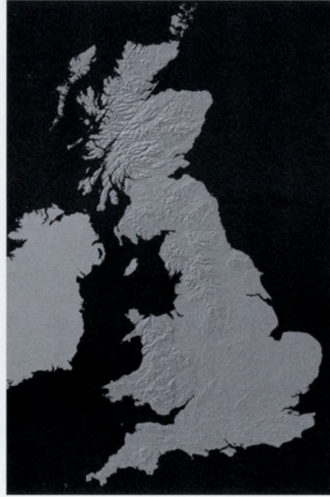
Digital Elevation Model of Great Britain. This image is a mosaic of over 2,800, ten-by-ten kilometre tiles of the digital surface model. It has been resampled from the original 5-metre postings to 50-metre postings and shaded to highlight relief.
